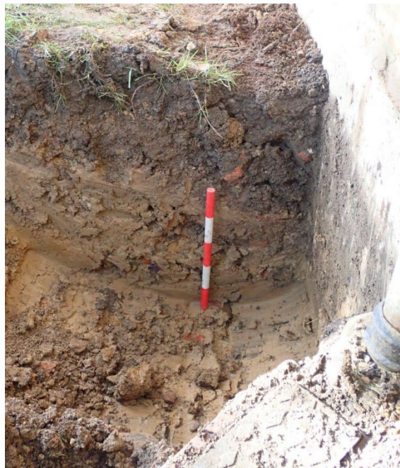
Plate 5: Pit looking west showing reworked clay [1] and natural clay [2] at base.
