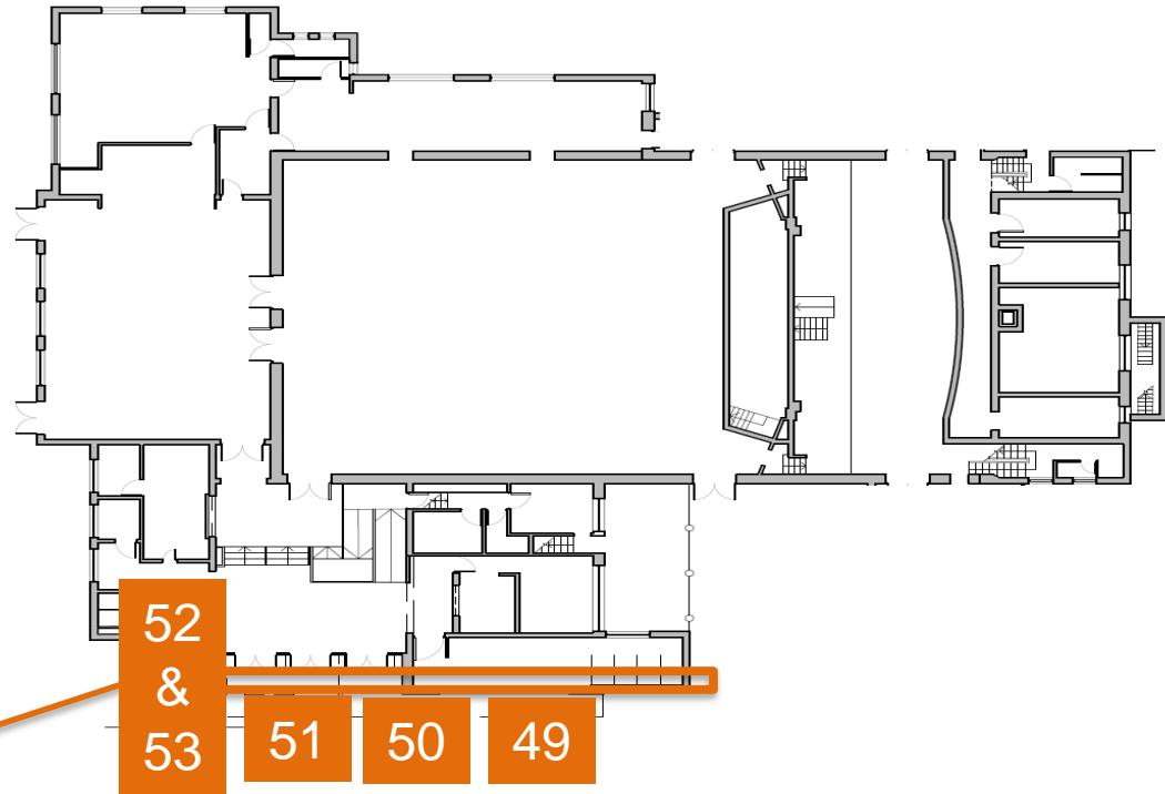
For the Supply and fitting of 5 No. of Secondary Glazing Windows (2 items as a two-part bay assembly), in white anodised aluminium finish, Hinged panels, 4mm Toughened glass, including latch locks and Seal tapes, to suit existing frames.
