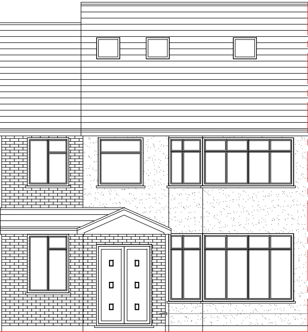
Proposed Rear Elevation (no.17) Scale 1:100
