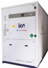
All i-Chiller components are selected with reliability and performance in mind. The advanced iC660 features a highly efficient, energy saving hermetic scroll compressor, its cutting edge evaporator provides high flow rates with low pressure drops and ultimate flexibility to tolerate return temperatures as high as 35°C or deliver glycol solution as low as -10°C. Furthermore the cold water tank keeps outlet temperature consistent despite varying loads conditions
