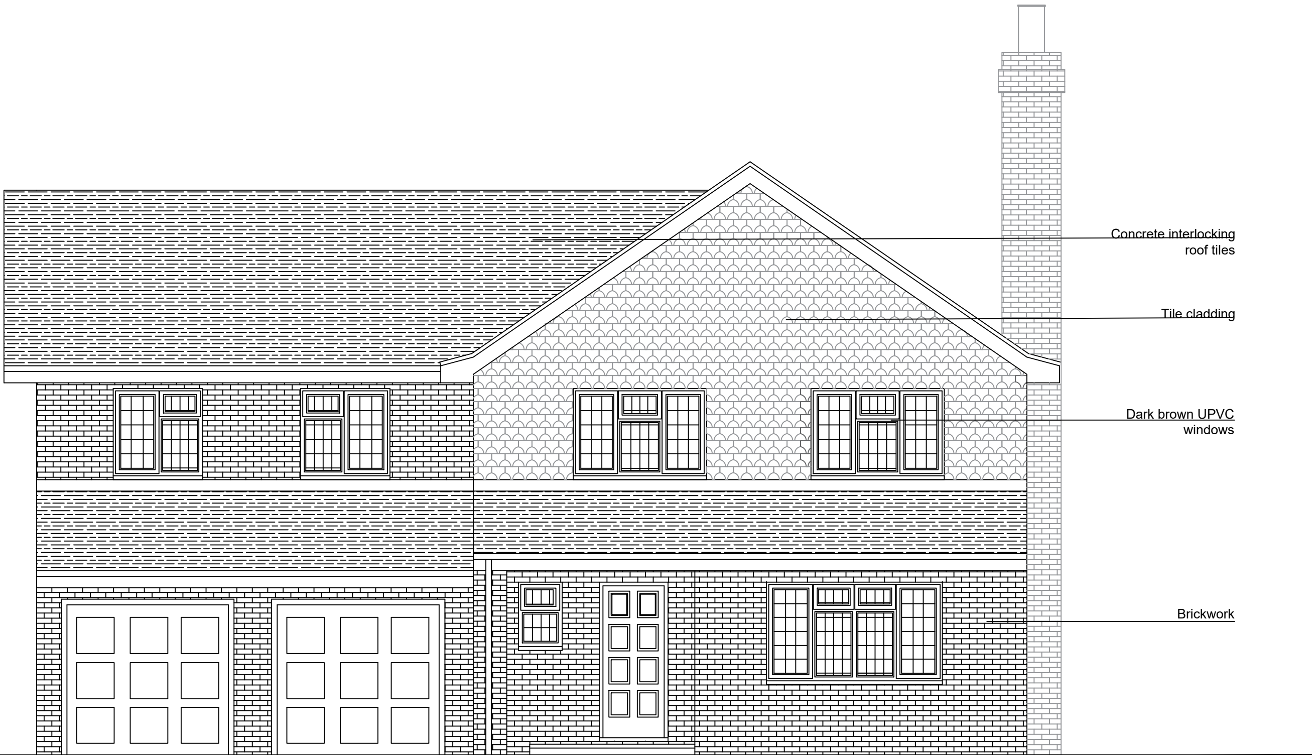
ELEVATION A EXISTING FRONT ELEVATION
