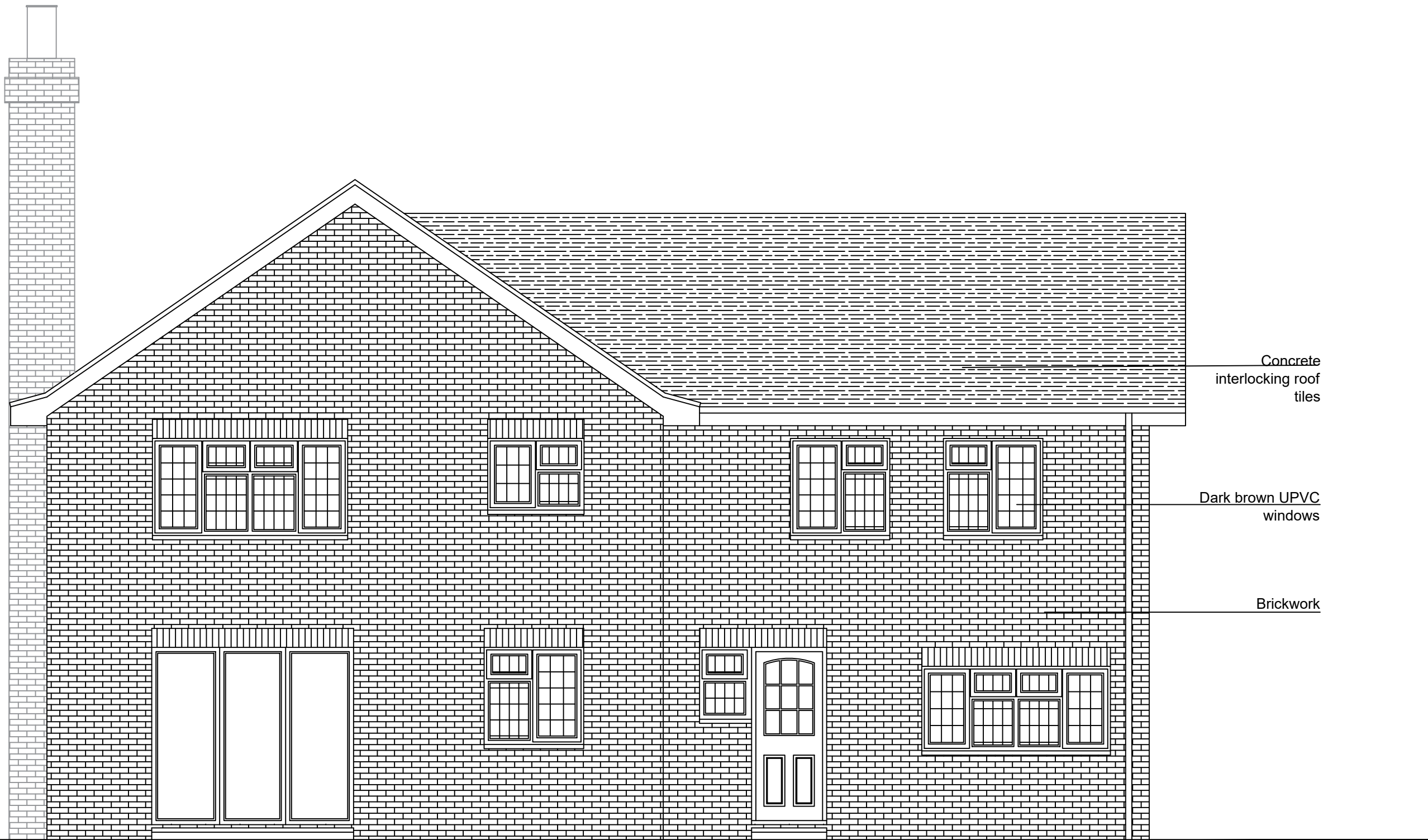
ELEVATION C EXISTING REAR ELEVATION
