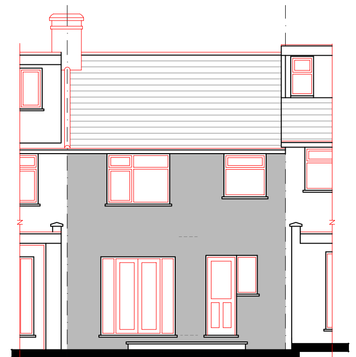
EXISTING REAR ELEVATION
