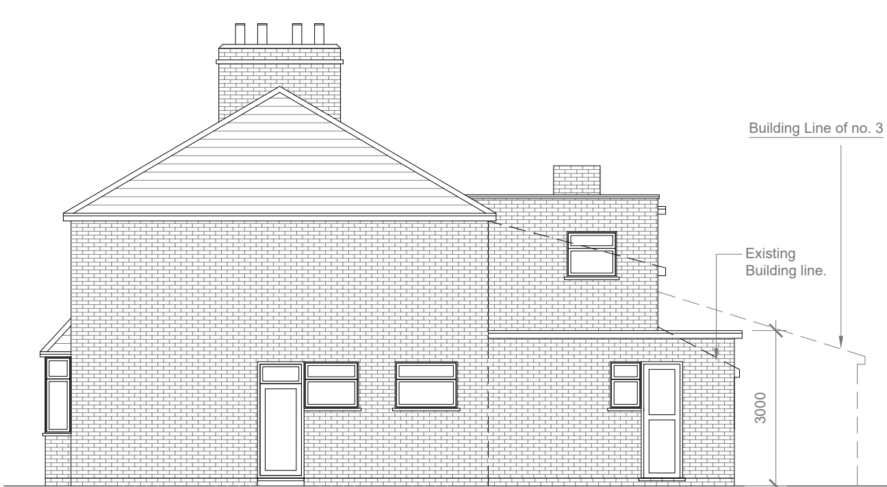
Proposed Side Elevation Scale 1:100
