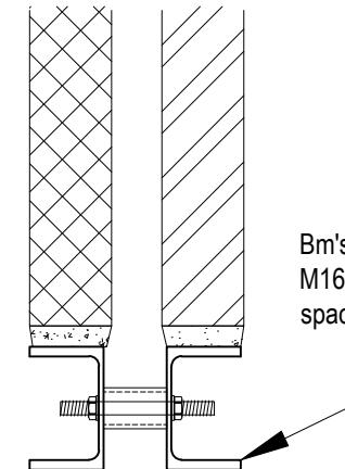
Bm's G1 and G2 bolted together with M16 threaded rods/washers/50Ø spacer tubes at 600 c/c.
