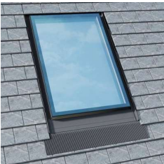
Slim line frame for pitched roof. Reset within roof tiles. Can be fixed to roof pitch as low as 12 deg. & as high as 90 deg.
