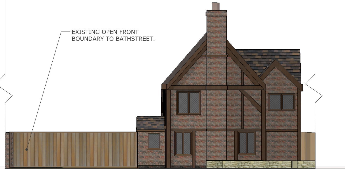
EXISTING FRONT STREET ELEVATION SCALE 1:100 @ A3
