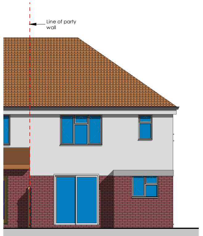
5 Rear Elevation (Existing) 2312-A-200 1 : 100
