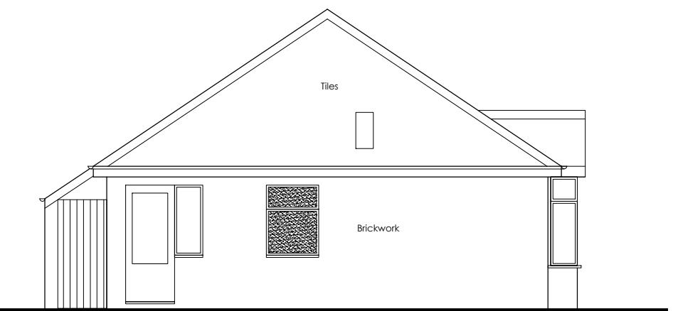
EXISTING WEST SIDE ELEVATION - Scale 1:100
