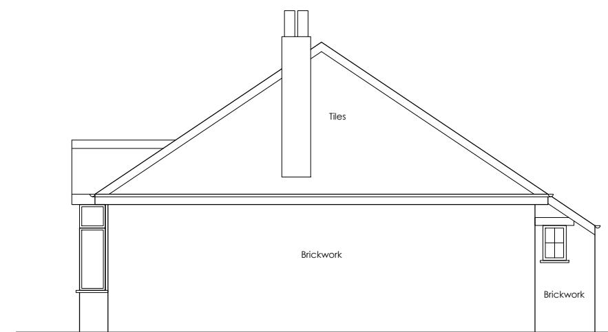
EXISTING WEST SIDE ELEVATION - Scale 1:100
