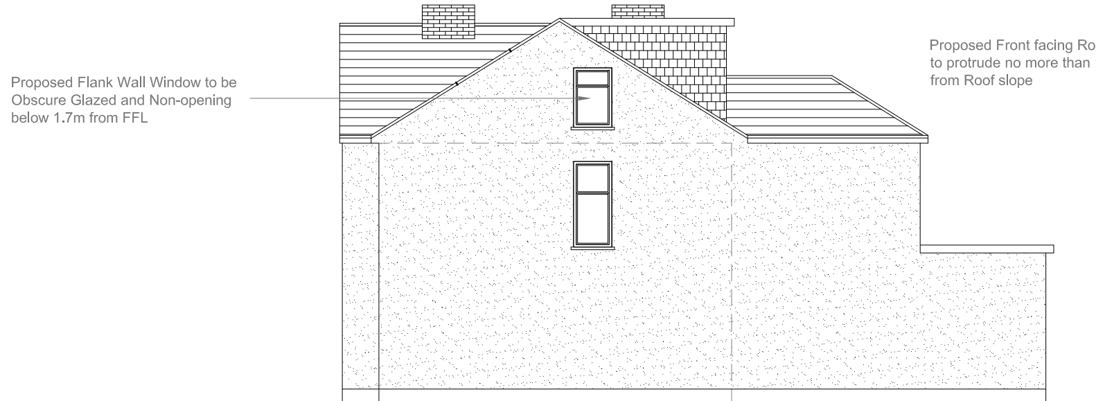
Proposed Side Elevation Scale 1:100
