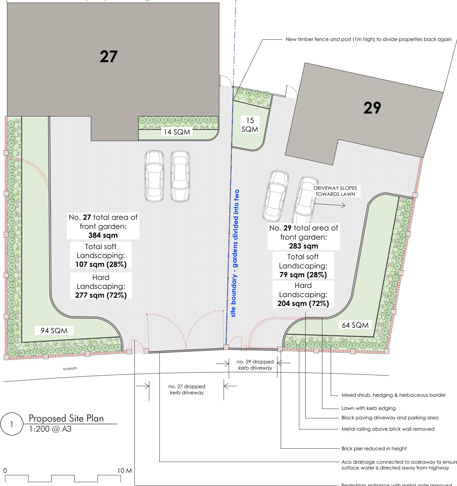
Dotted red lines indicate existing to be demolished or reduced in height
