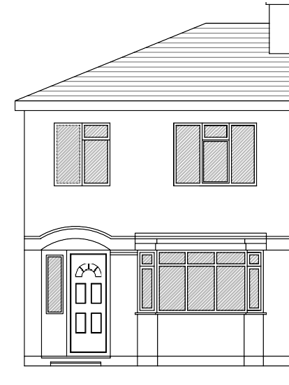
EXISTING FRONT ELEVATION 1:100
