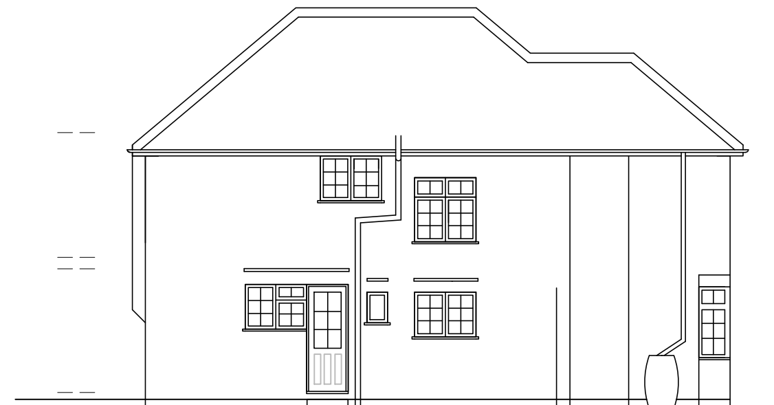
EXISTING SIDE ELEVATION TO WEST SCALE 1:100
