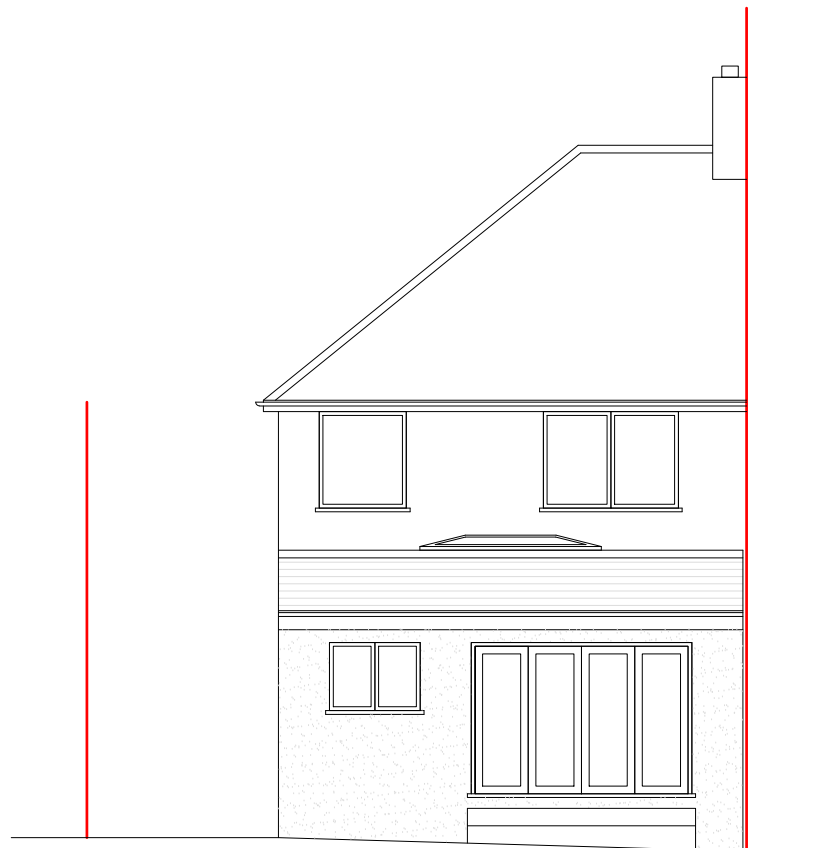
Proposed Rear Elevation Scale:1:100
