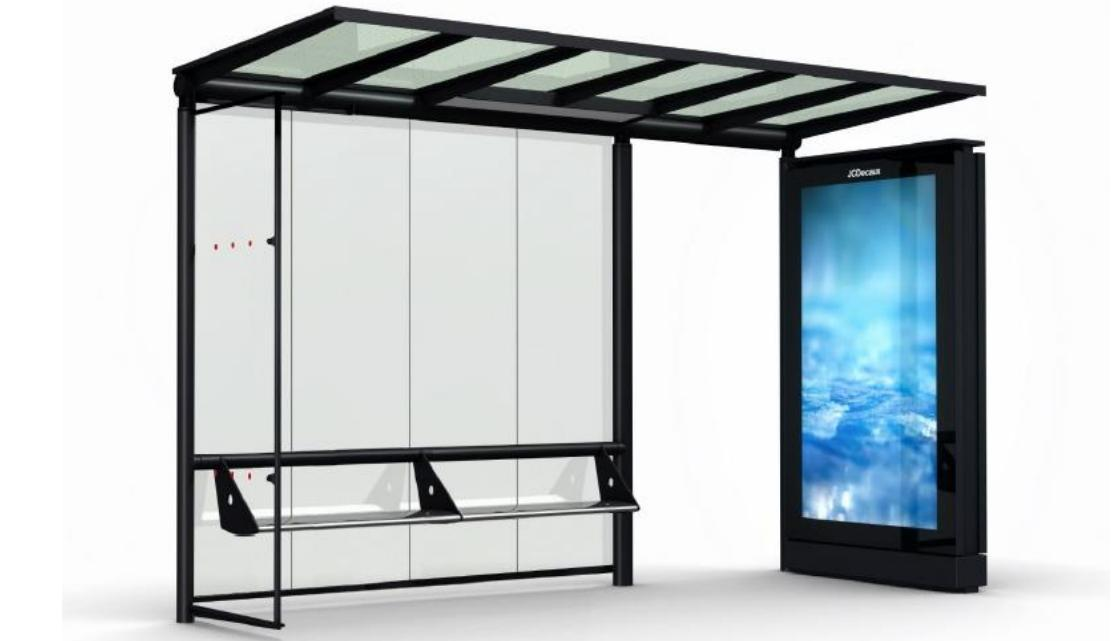
The shelter roof structure is welded steel construction, supporting five panels of toughened laminated glass, which cannot fall in the event of breakage. The glass is specially treated to reduce the heat of the sun rays by more than 50% and is waterproofed through seals fitted in the glazing bars. The shelter roof is gently sloped to drain rainwater behind rear glass.
