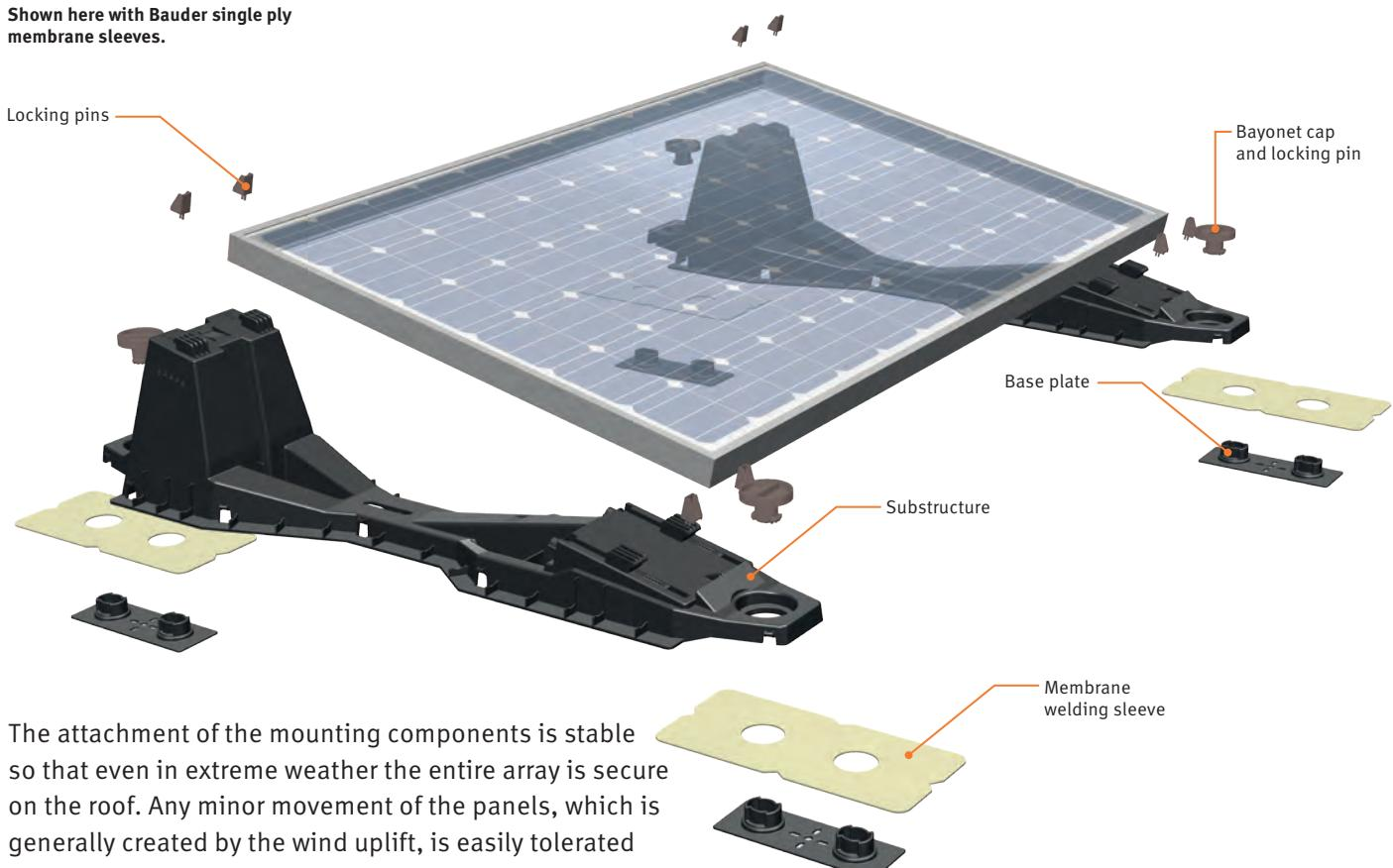
The attachment of the mounting components is stable so that even in extreme weather the entire array is secure on the roof. Any minor movement of the panels, which is generally created by the wind uplift, is easily tolerated and has minimal affect on the fixings or waterproofing system.
