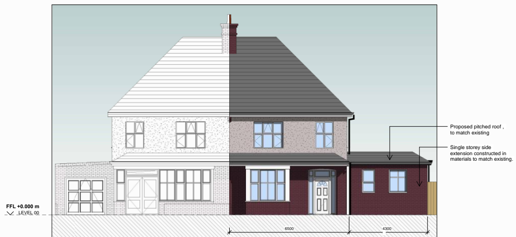
1 FRONT ELEVATION - AS PROPOSED 1:100
