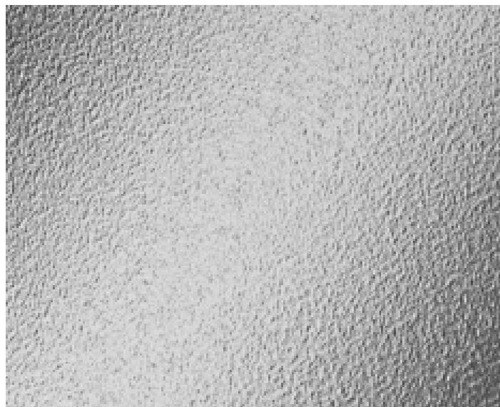
Obscure Glass at minimum 1.7m from Finish Floor Level (Stippolyte Type) to First floor rear and side elevation windows.
