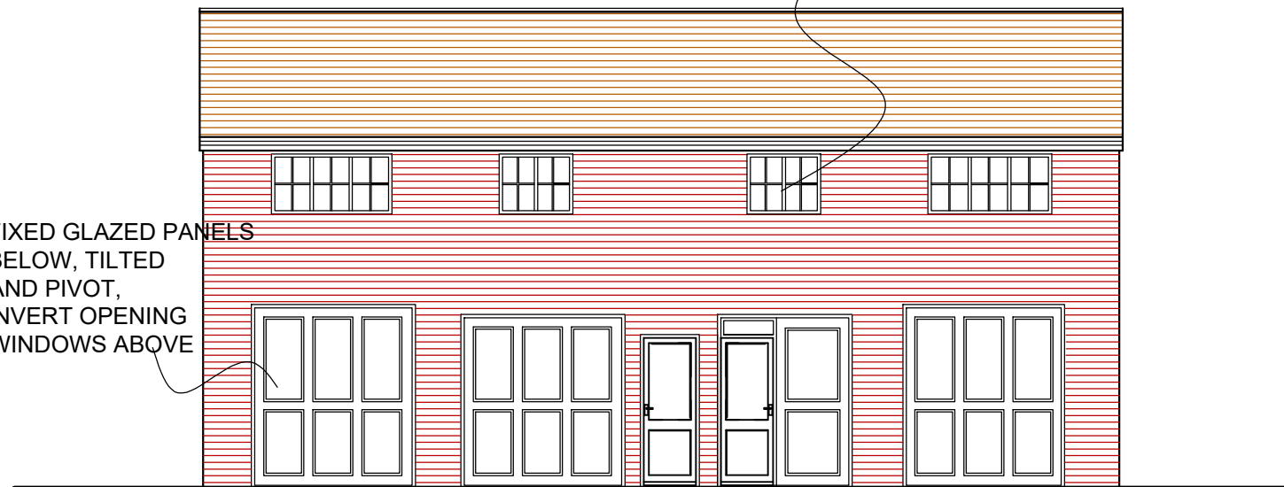
SOUTH WEST ELEVATION
