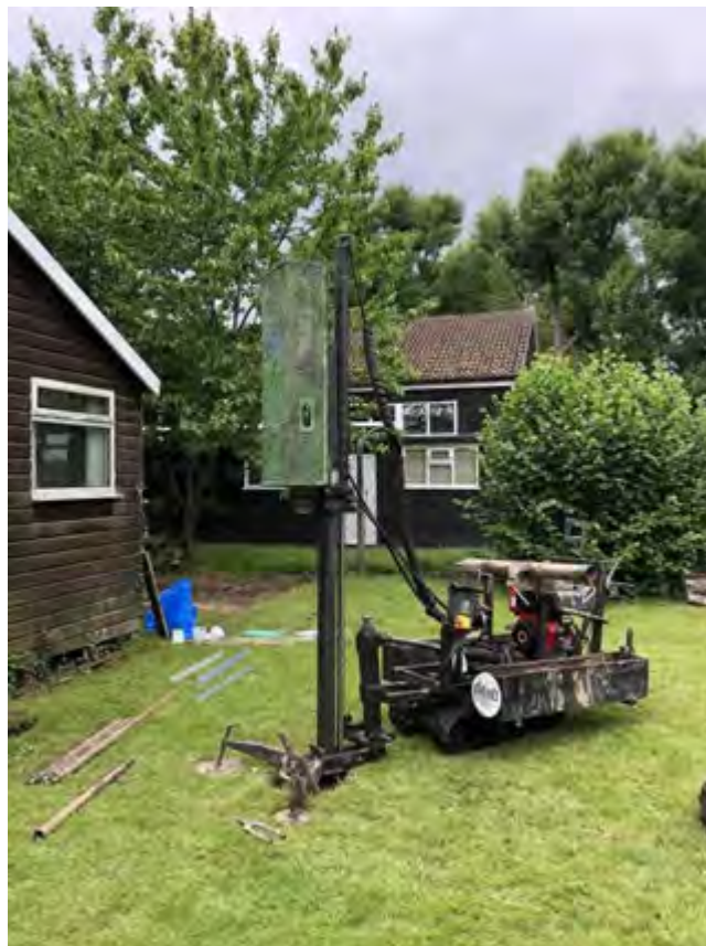
Photograph 10: Dando Terrier Rig used for drilling works (photo taken at WS04).
