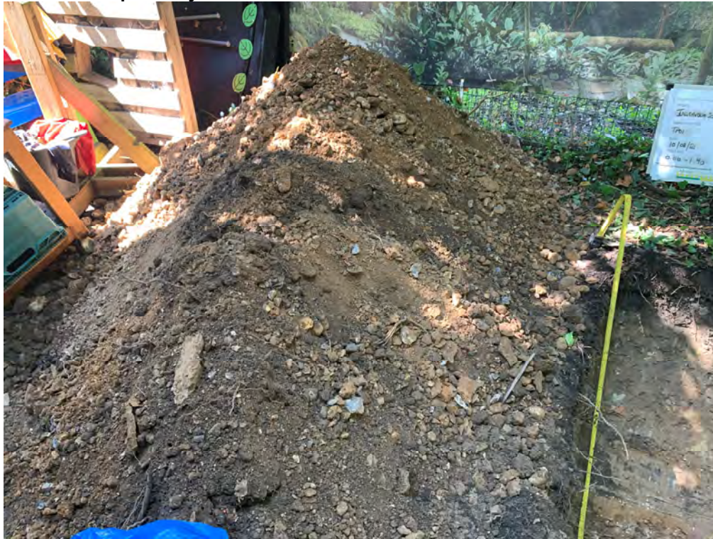
Photograph 3: Encountered spoil materials. TP01 0.0 – 1.9mbgl.
