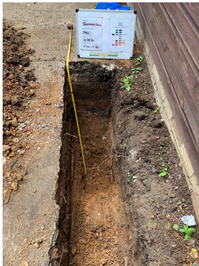
Photograph 4: Encountered ground materials. TP02 0.0 – 1.6mbgl.
