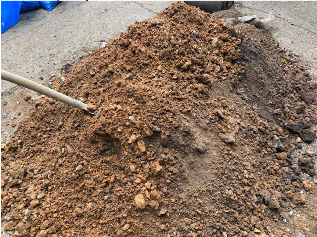
Photograph 5: Encountered spoil materials. TP02 0.0 – 1.6mbgl.
