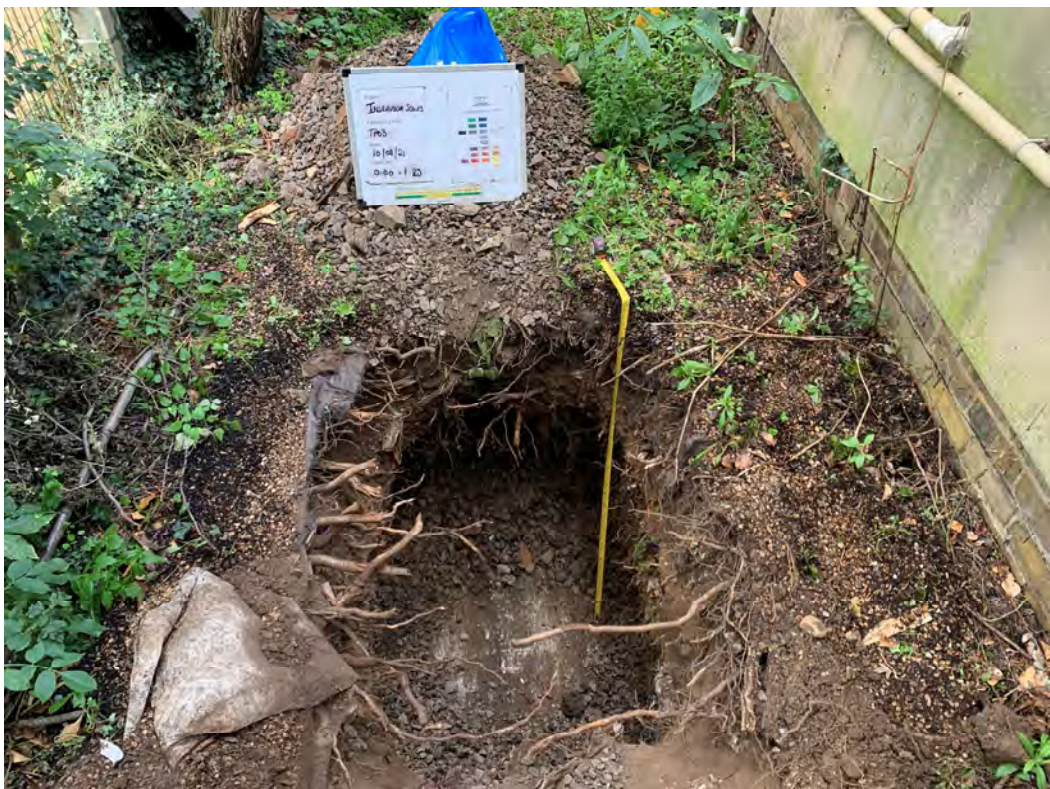
Photograph 6: Encountered ground materials. TP03 0.0 – 1.3mbgl.
