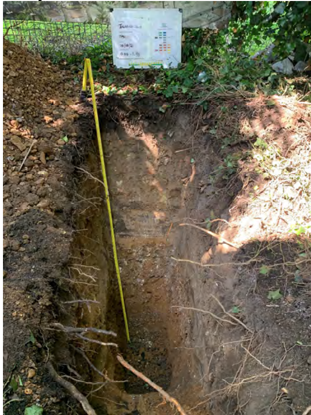
Photograph 1: Encountered ground materials, TP01. 0.0 - 1.9mbgl
