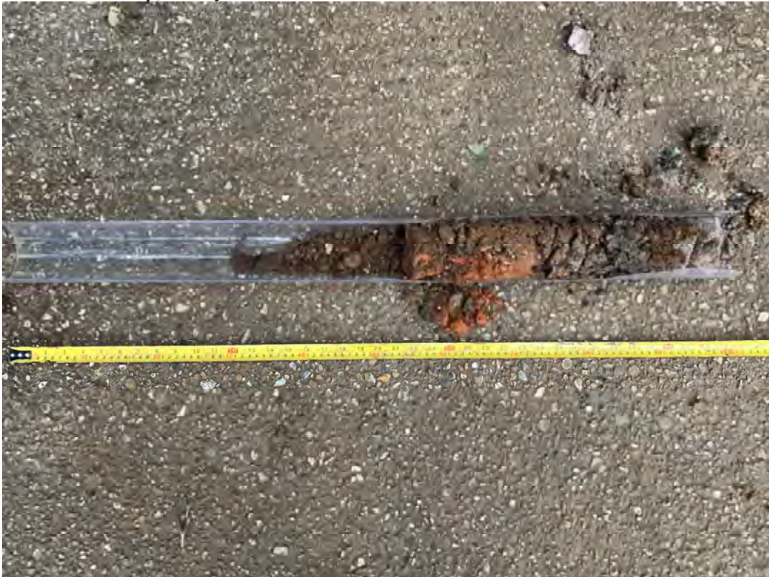
Photograph 7: Encountered ground conditions. WS05 0.0 – 1.0mbgl.
