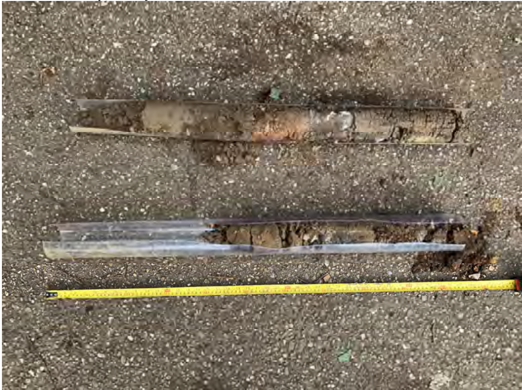
Photograph 5: Encountered ground conditions. WS03 0.0 – 1.6mbgl.
