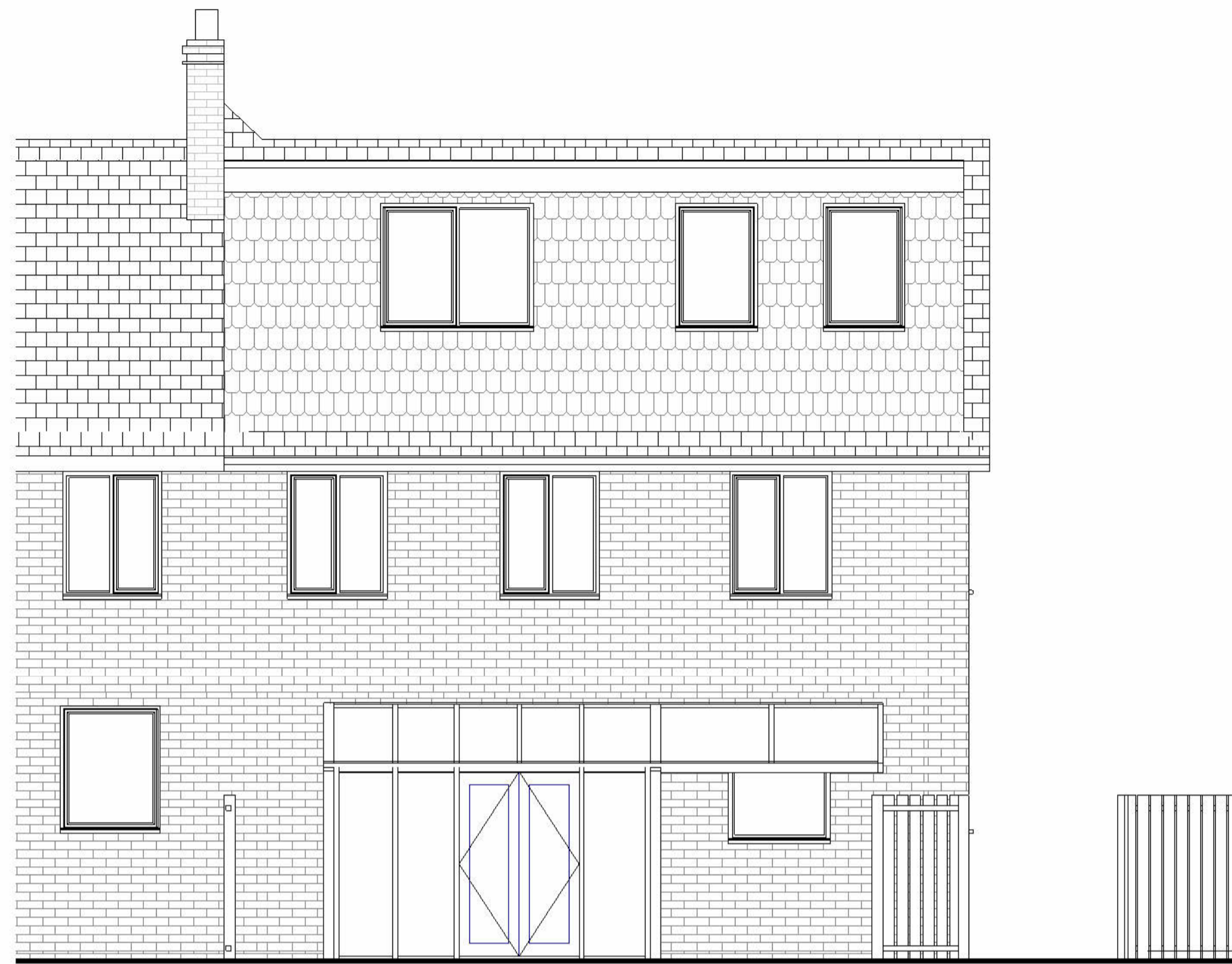
2 Rear Elevation 1 : 50 (Existing)
