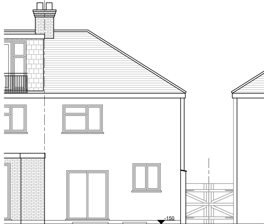
EXISTING REAR ELEVATION SCALE 1:100
