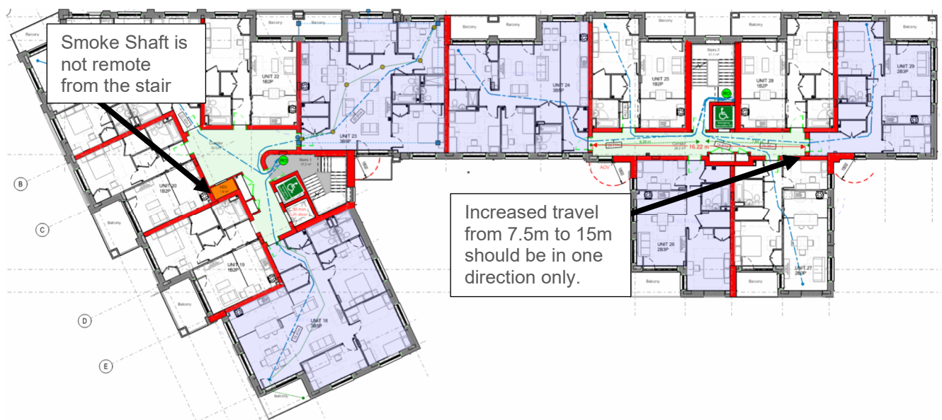
Figure 17: Smoke ventilation protection to stairs
