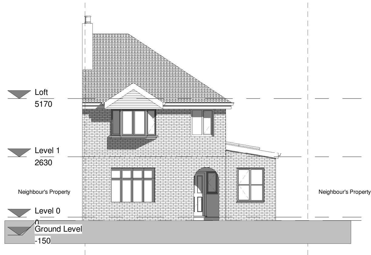
1 Front elevation - Existing 1 : 100
