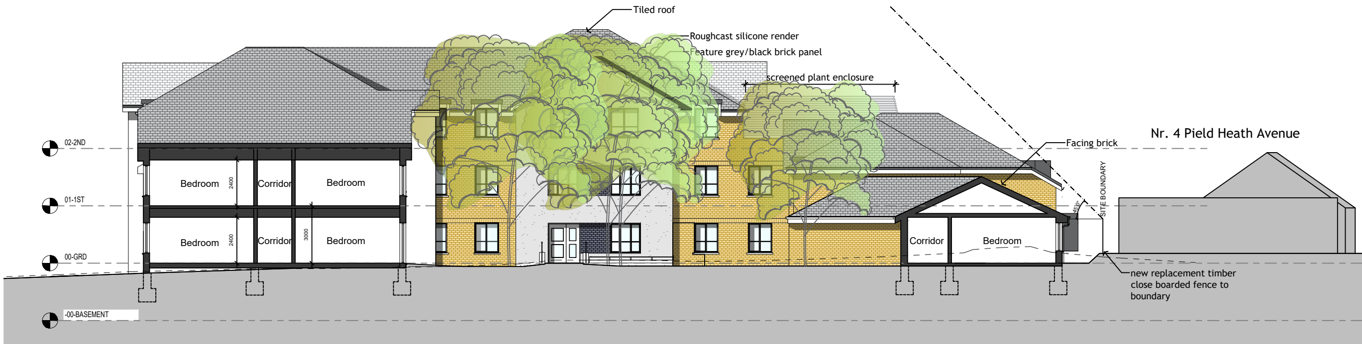
Part Section A-A: North-East facing elevation (1:200)
