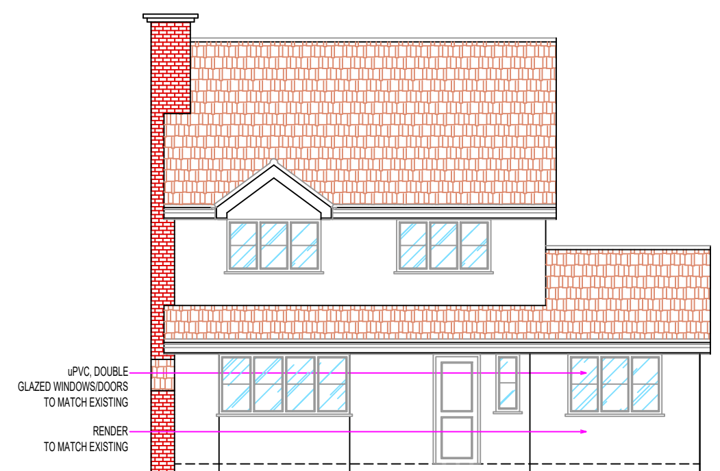
PROPOSED FRONT ELEVATION SCALE 1:100@A1
