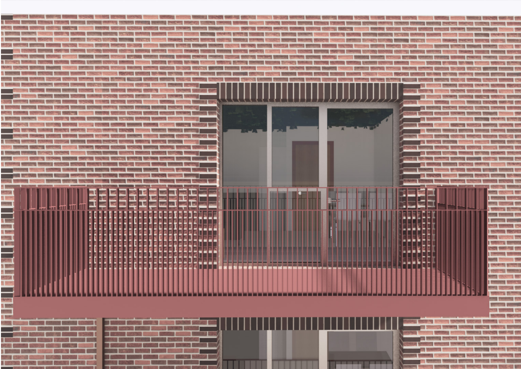
Elevation view of projecting railing balcony
