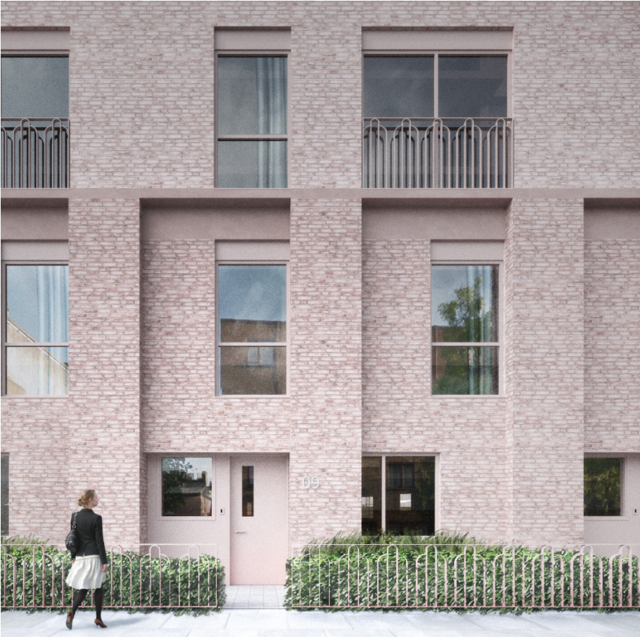
Brick detailing to define duplex homes (Ashley Road West, PTE)
