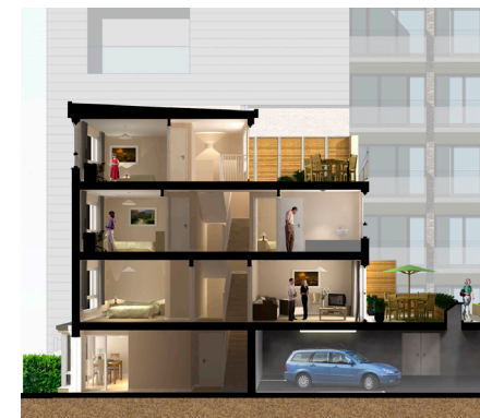
Podium parking integrated within the block design with active frontage along the street
