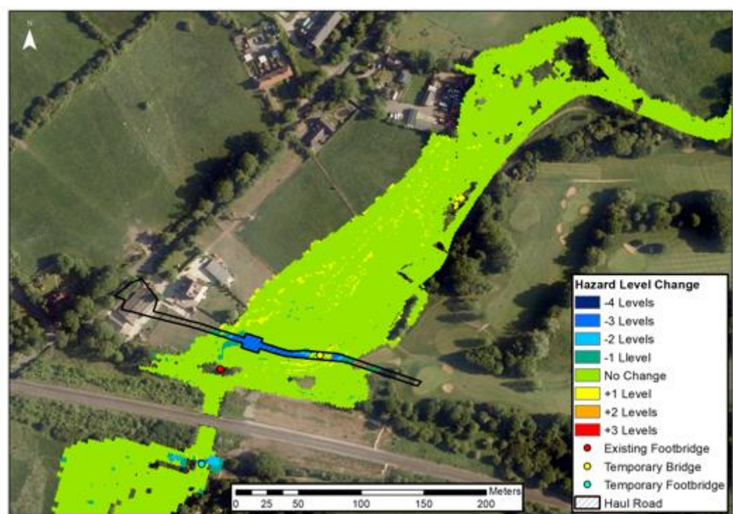
Figure 14 Hazard level change between Baseline and Scenario 1 for T30 return period.
