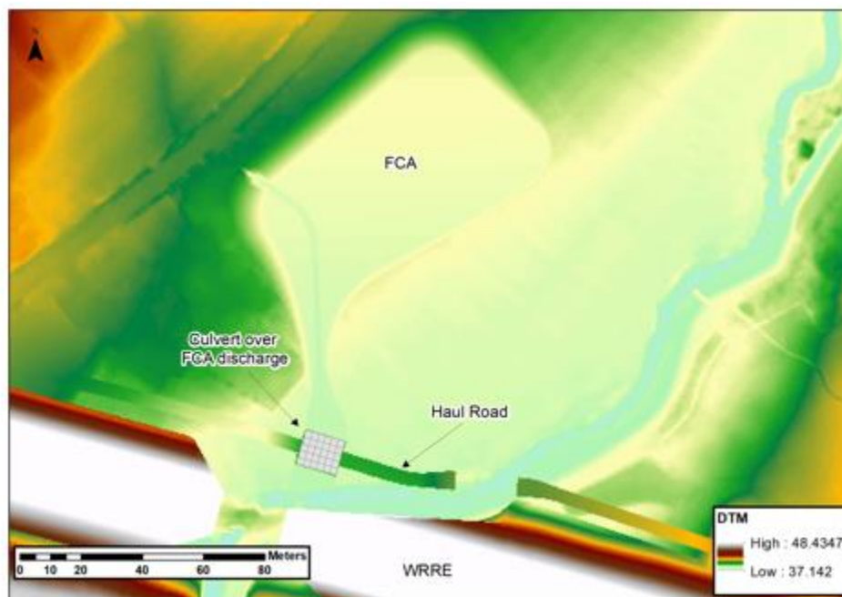
Figure 8 Culvert structure position. (DTM in m AOD).
