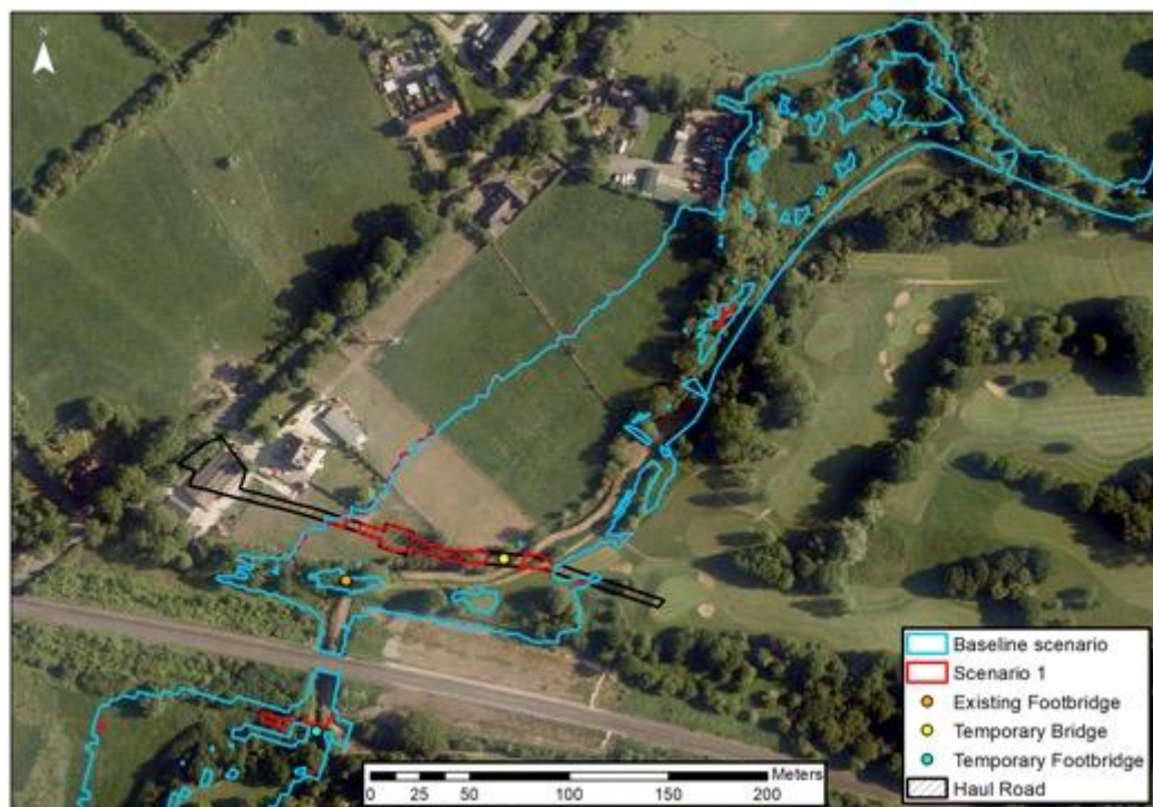
Figure 12 Flood extent comparison between Baseline and Scenario 1 for T30 return period.
