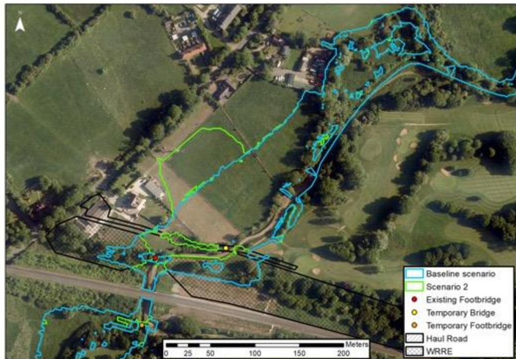
Figure 15 Flood extent comparison between Baseline and Scenario 2 for T30 return period.
