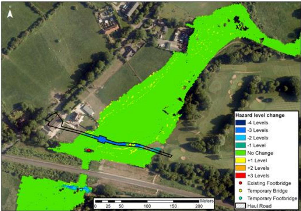
Figure 23 Hazard level change between Baseline and Scenario 1 for T100 return period.
