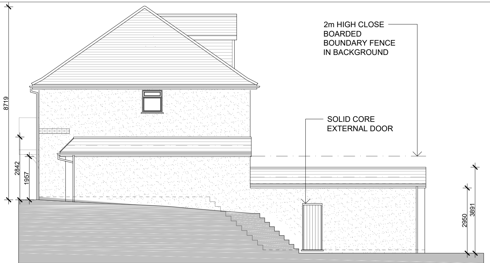
SIDE (SOUTH WEST) ELEVATION
