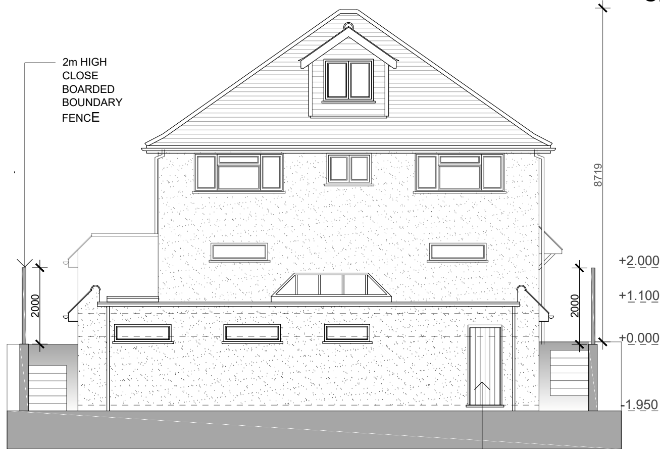
REAR (SOUTH EAST) ELEVATION
