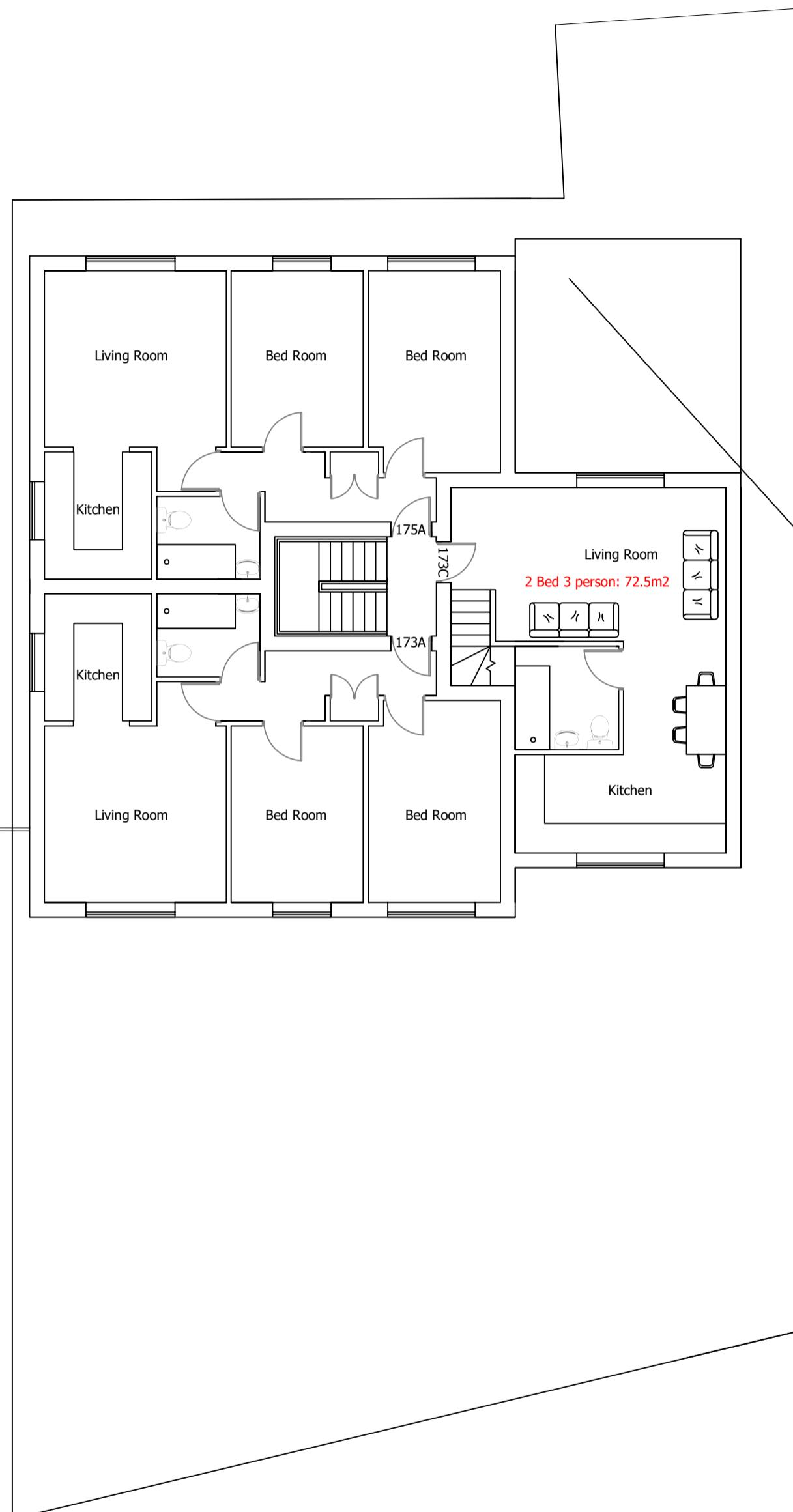
Drawing: Proposed First Floor Plan Scale: 1:100 (A3)
