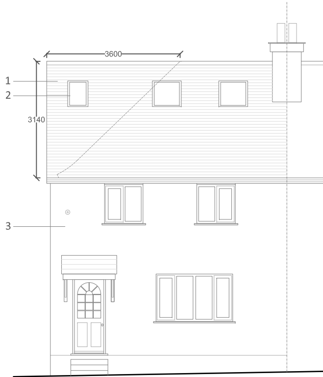
Proposed Front Elevation SCALE 1:100
