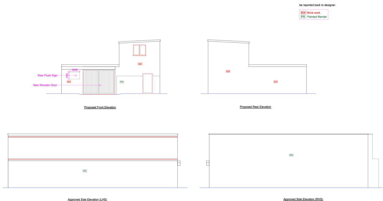
The current application seeks a **variation to these approved plans**, specifically to allow the replacement of the approved timber doors with a **roller shutter**, as illustrated in the updated plans:
