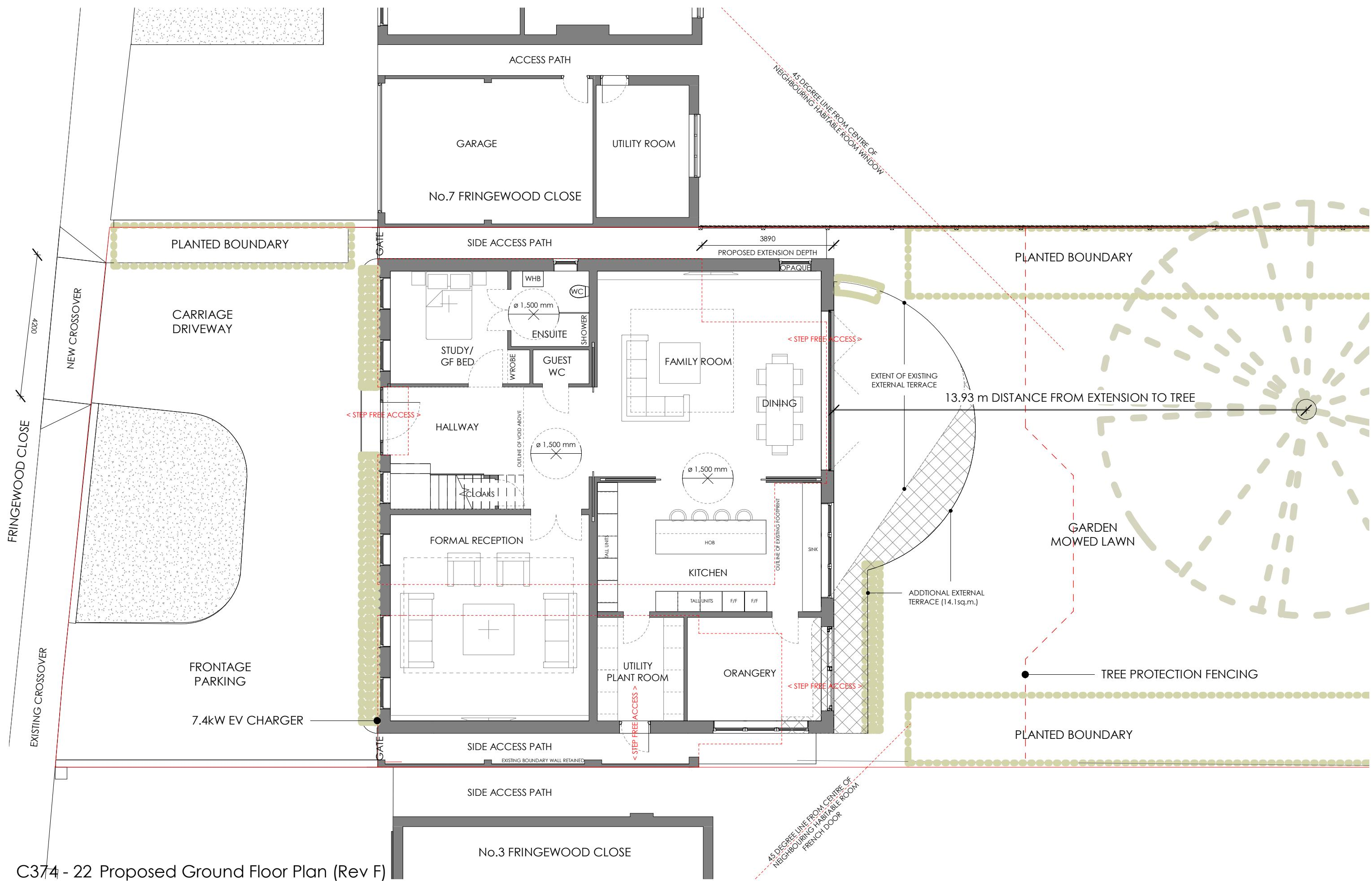
C374 - 22 Proposed Ground Floor Plan (Rev F)
