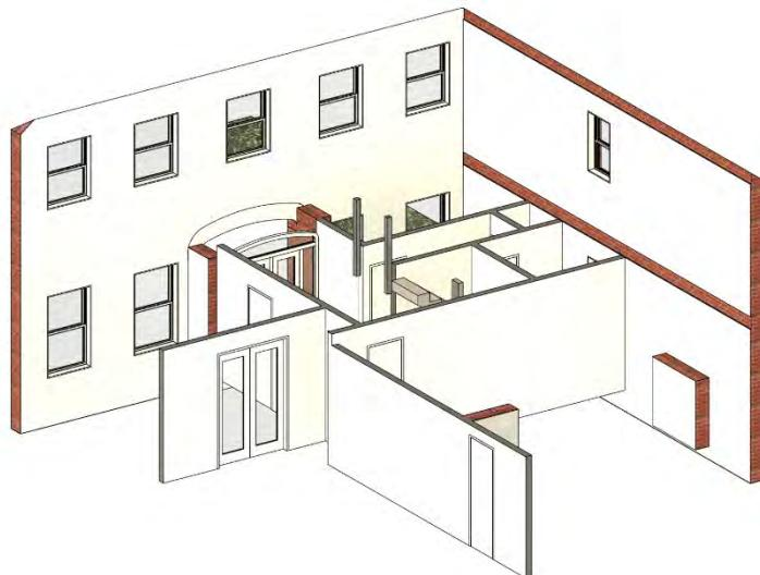
The consented drawings show how the ground floor internal walls need to be removed. The existing floor needs to be removed to install a ground floor that meets current insulations standards.
