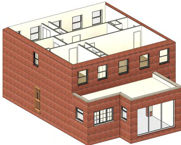
To construct the extension to the front reception room, the garage, built of single skin brickwork, needs to be demolished.
