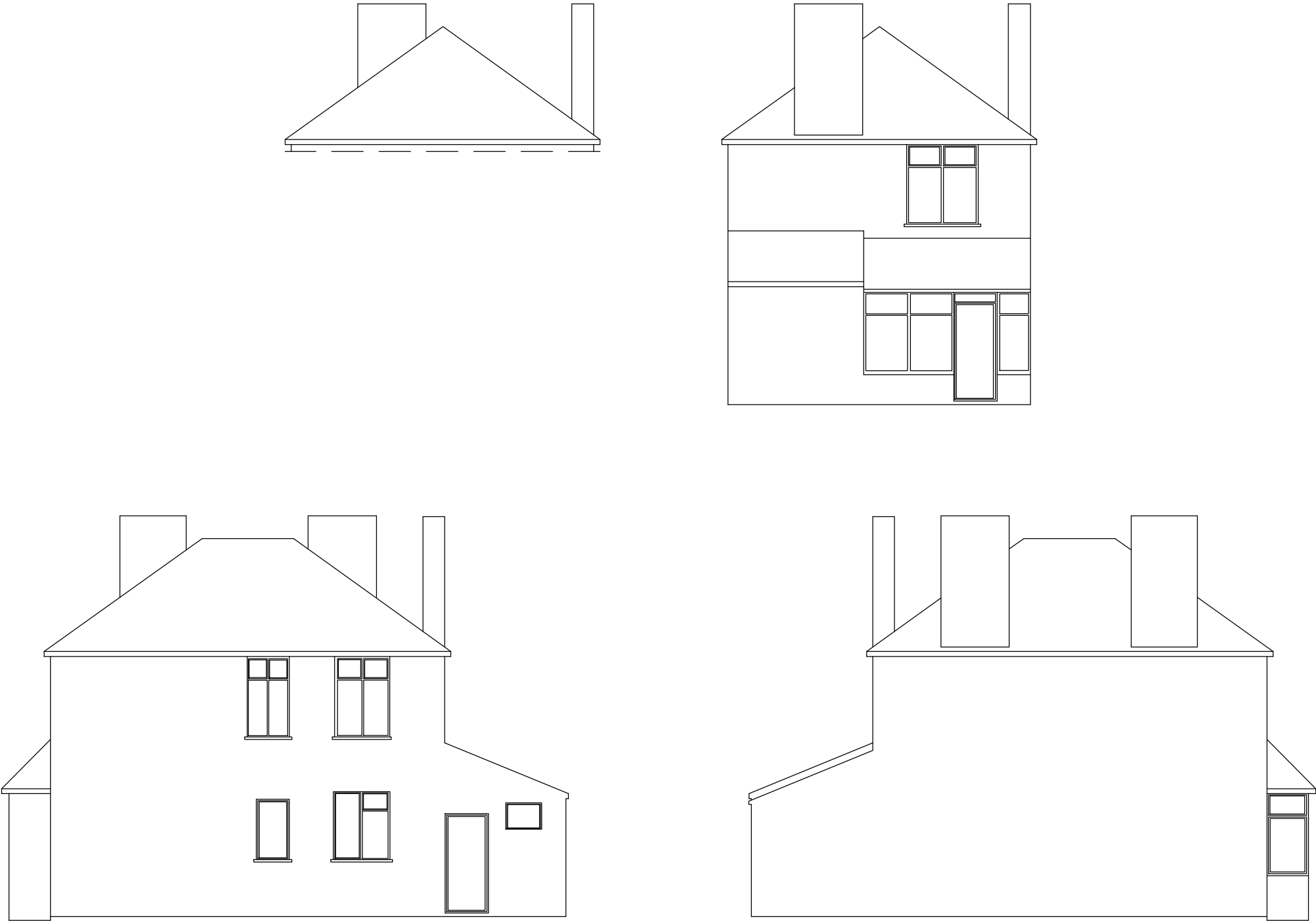
EXISTING PART FRONT / REAR & SIDE ELEVATIONS Scale 1:100
