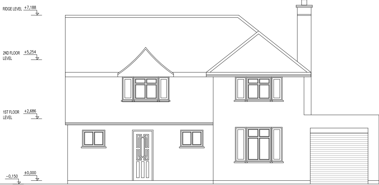
EXISTING FRONT ELEVATION 1:100
