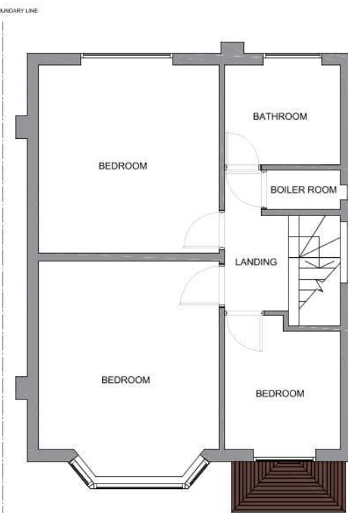
FIRST FLOOR (existing) Scale 1:100
