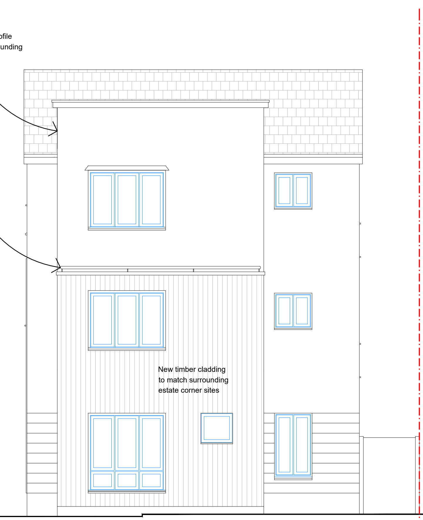
PROPOSED FRONT ELEVATION SCALE 1:50
