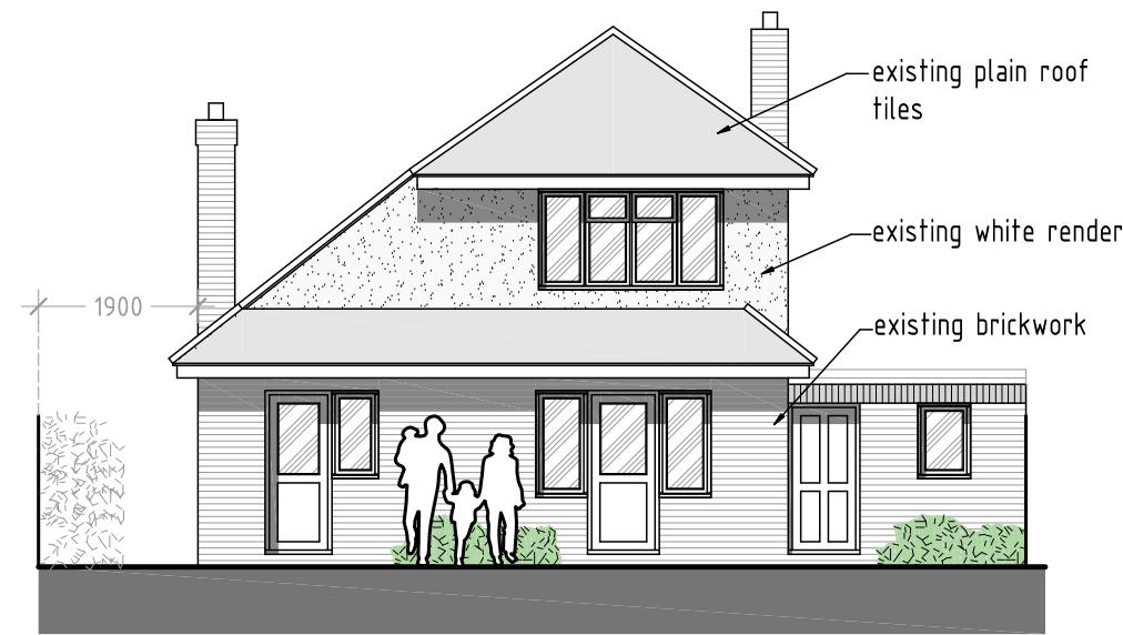
EXISTING REAR ELEVATION - 1:100
