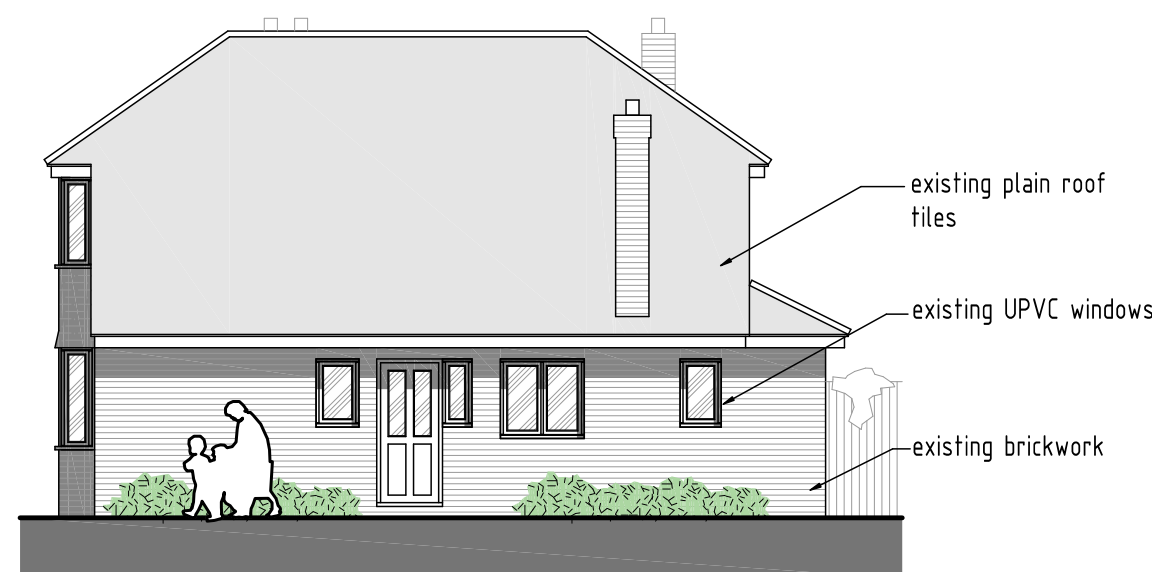
EXISTING SIDE ELEVATION - 1:100
