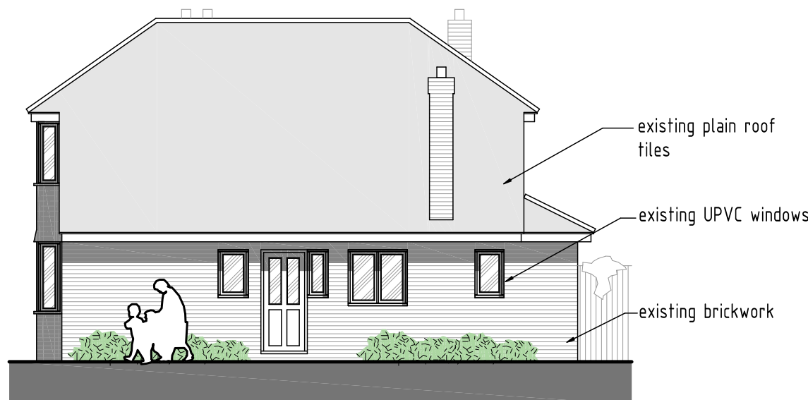
EXISTING SIDE ELEVATION - 1:100
