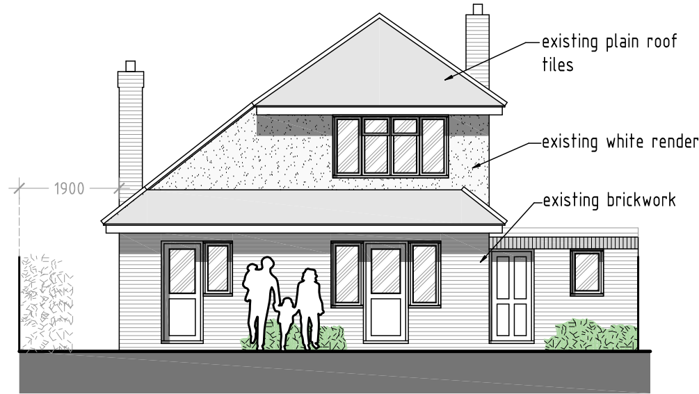
EXISTING REAR ELEVATION - 1:100
