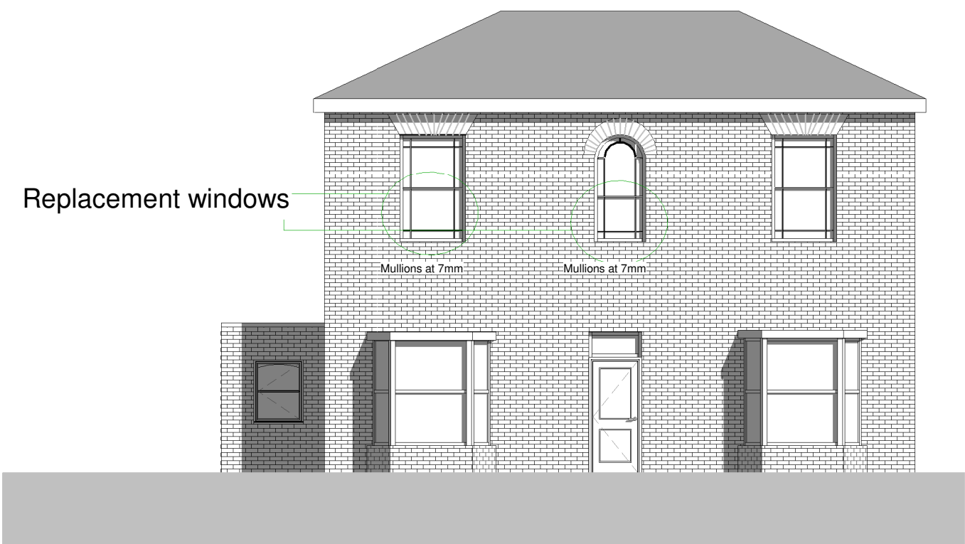
Front elevation - Proposed 1 : 100
