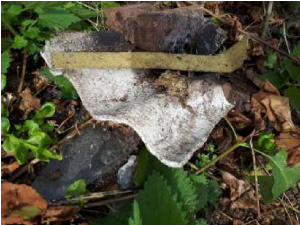
Plate 10: Potential asbestos containing material (ACM).
